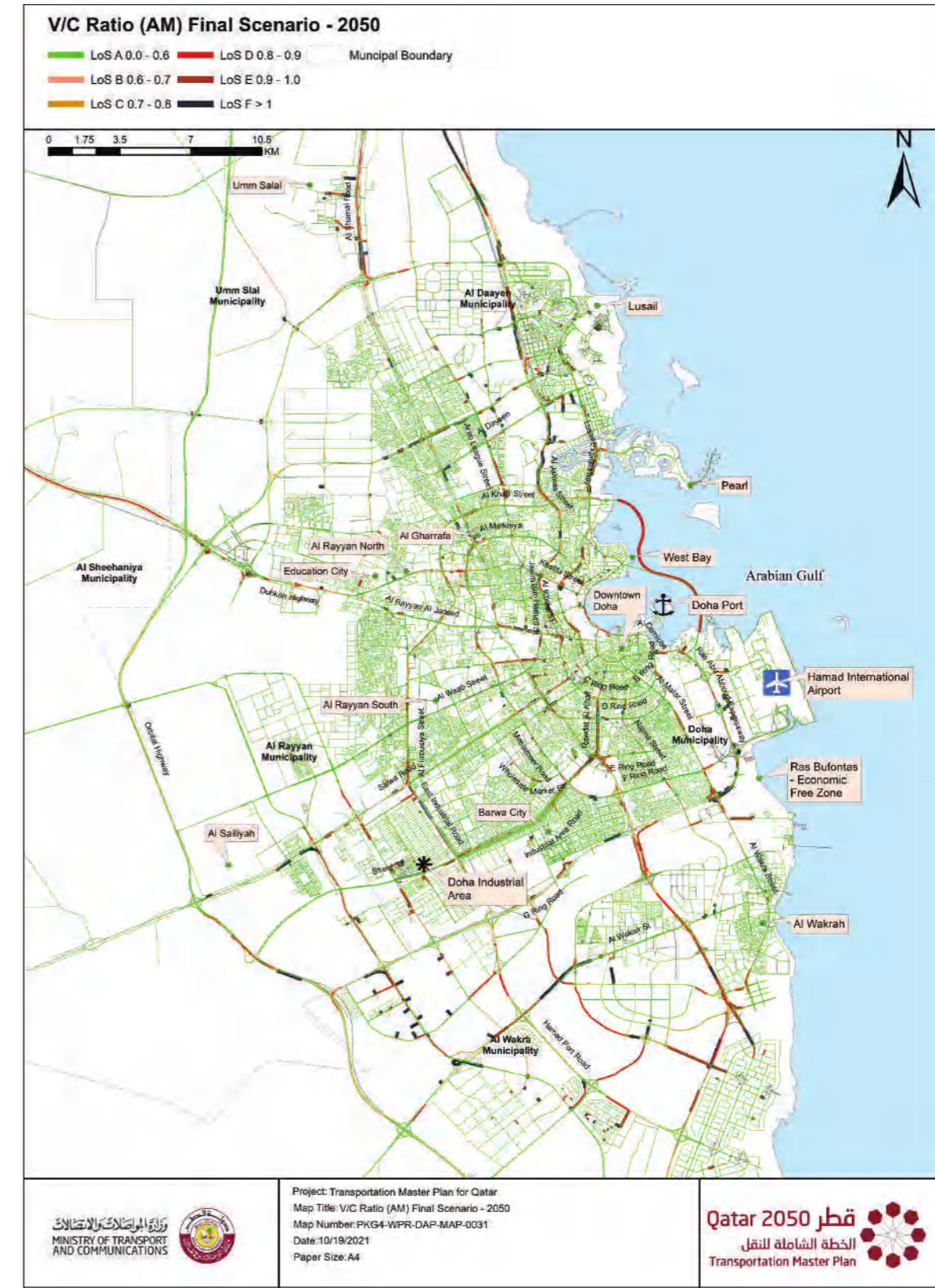
Levels of Service (V/C) for the AM Peak in the Updated TMPQ, Doha (2050)
