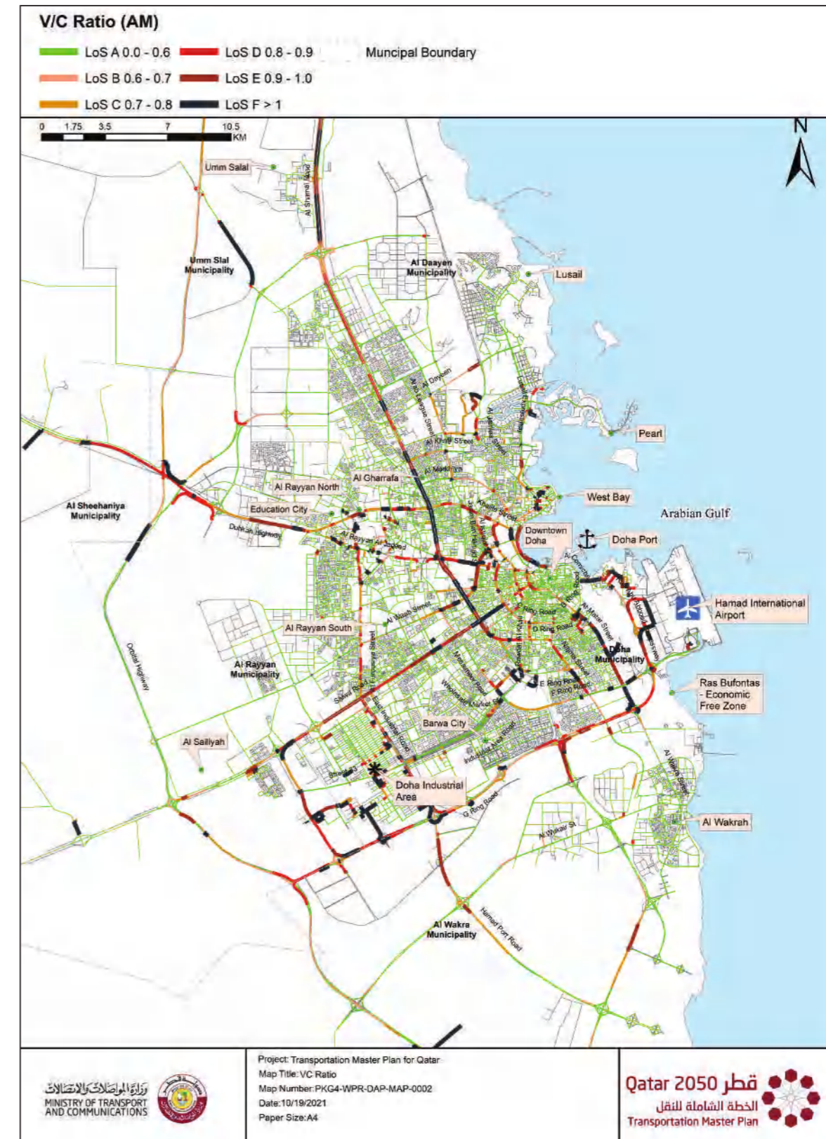
Existing Congestion Levels on Main Roads Within DMA during Morning Peak Hour
