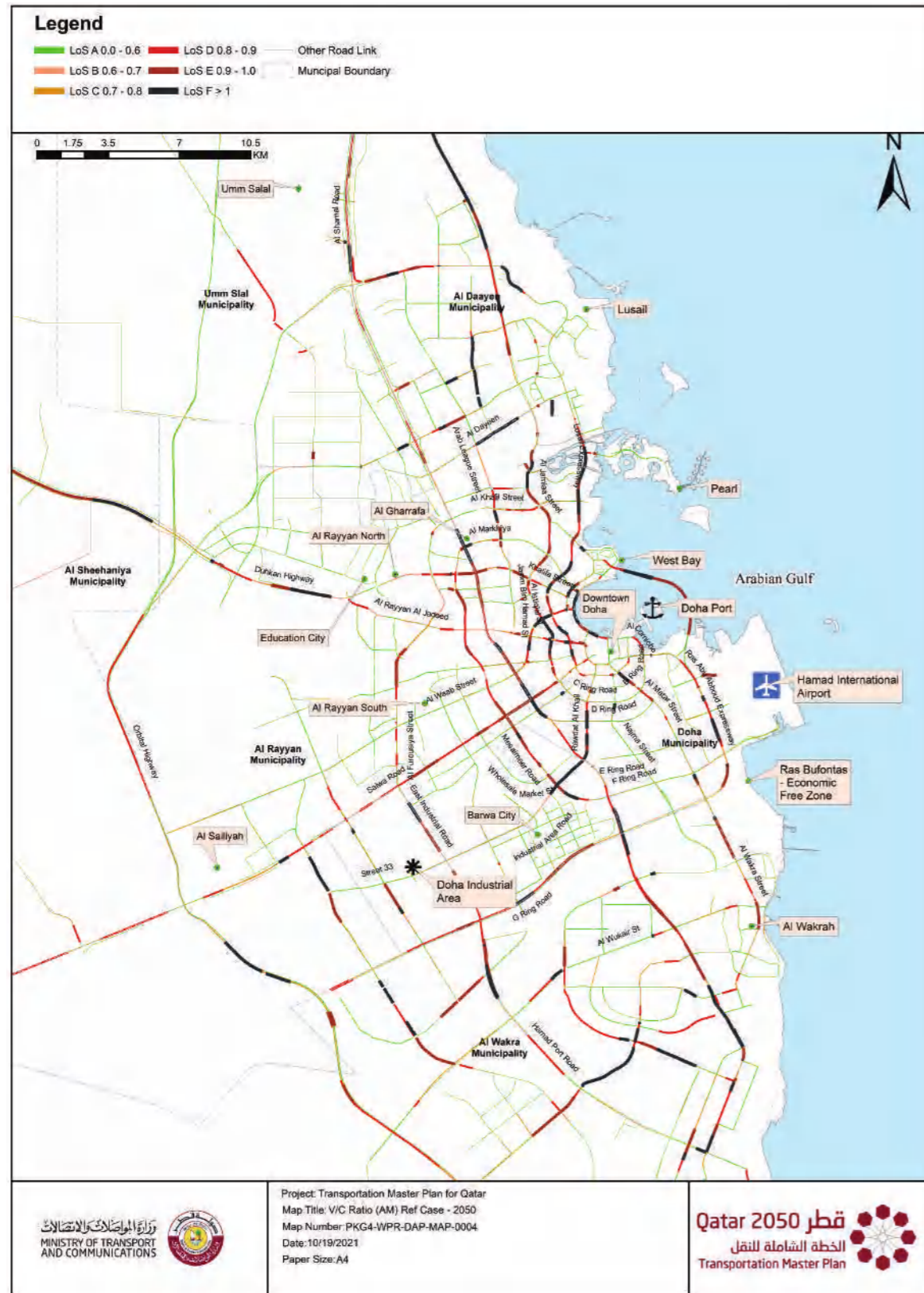
Congestion Levels on Main Roads Within DMA during Morning Peak Hour (2050 Reference Case)
