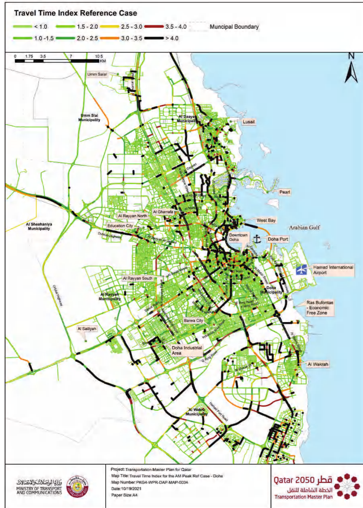
Travel Time Index for the AM Peak in the Reference Case, Doha (2050)
